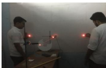
Figure 4: A laser beam reflecting from the rulings of an audio compact disk and producing a diffraction pattern on a screen.
