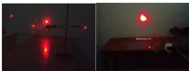
Figure 5: A laser beam transmitting from the rulings of an audio compact disk (left) and DVD (right) and producing a diffraction pattern on a screen.
