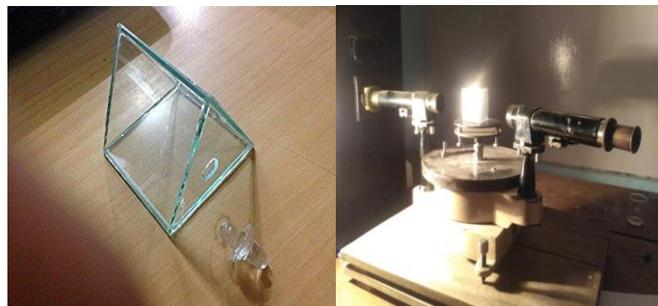
Figure 3: (a) Hollow glass prism (b) Experimental set up for analysis of refractive index of different concentrated solutions.
