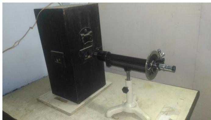
Figure 2: Experimental set up for measurement of angle of rotation for different solutions.
