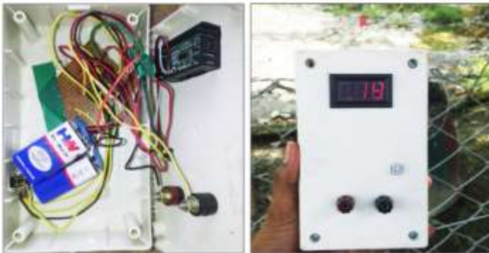
Fig. 2: The self-constructed Sun Photometer designed for the work- Internal circuitry and external view
