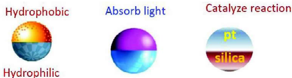
Figure 1: Schematic of spherical Janus particles with two distinct hemispheres with different interaction with solvent (left one), light absorbing properties (middle one) and catalytic properties (right one).
