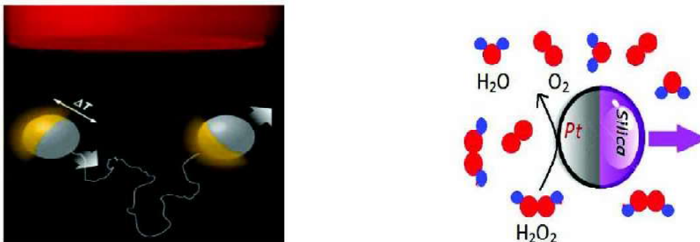
Figure 3: Schematic self-propulsion mechanisms. Left - Self-propulsion based on the thermophoresis. Right - diffusiophoresis is responsible for self-propulsion.
